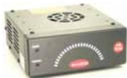
13.8 VDC, 14 Amp Surge 12 Amp Continuous, Light Weight, only 2.7 lbs!, Compact, only 6.5" x 5.75" x 2.25", Over voltage protection, Over current protection, Quiet internal cooling fan, Switchable AC input voltage, 115 or 230 Vac AC line fuse (3 amps for 230V, 6 amps for 115V)
